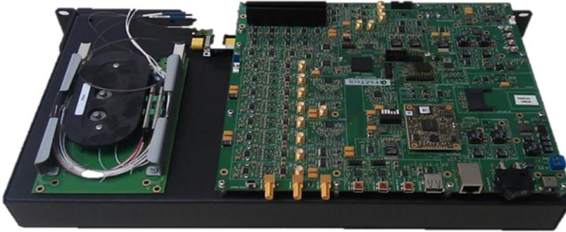
FAZ I4 Interrogator, optics (left) and electronics (right) boards
