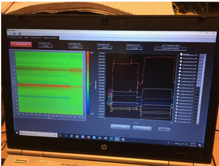
**Fig.9: Display of the FO Strain measurement system during Factory Acceptance Test. The left panel displays a complete pile as strain color map, the right panel gives conventional strain versus time display for a group of sensors.**
