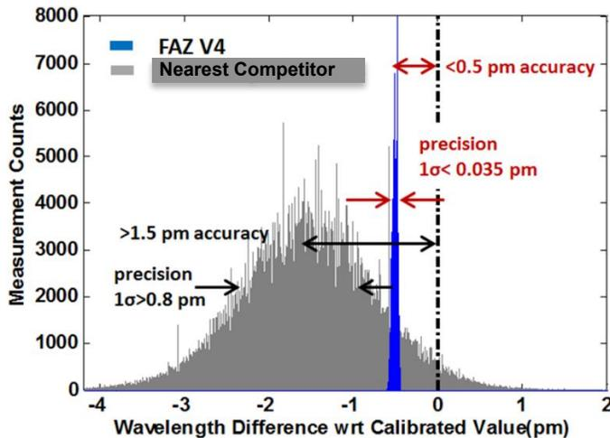
Fig. 3: FAZ I4, precision and accuracy compared to the nearest competitor ( [redacted] system). A single FBG under controlled conditions is measured for a long time, the individual measurements are sampled into a distribution. The deviation from the “true” measurement is defined as precision, the width of the distribution (the scatter) is defined accuracy.
