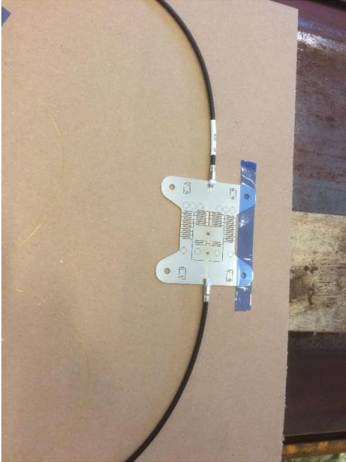
**Fig. 6: Fugro Strain sensor, basic sensing element without cover and protection. The combination of optical fiber and spring “multiplier” is clearly visible, the fiber runs between the two black cable ends across the spring structure and is mounted using mineral glass solder. The round “spots” are the markers for the actual welding points to the to be monitored structure.**
