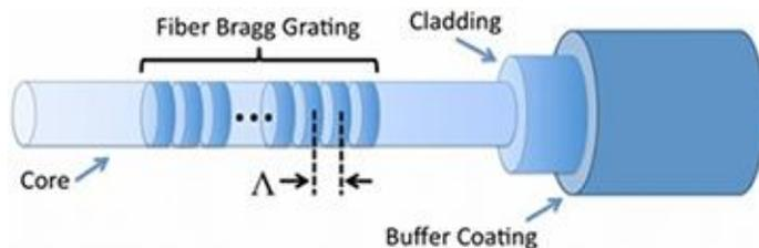
**Fig.1 Principle of a Fiber Bragg Grating.** A periodic change of the refractive index of the fiber is introduced. The Bragg condition based on the periodicity gives the selectively reflected wavelength. A change of the grating dimension/periodicity changes the reflected wavelength. Therefore, the FBG becomes a natural strain and temperature sensor.
