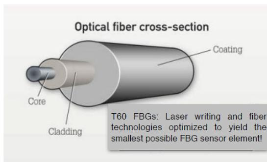
Fig.2. Optical fiber cross-section.
